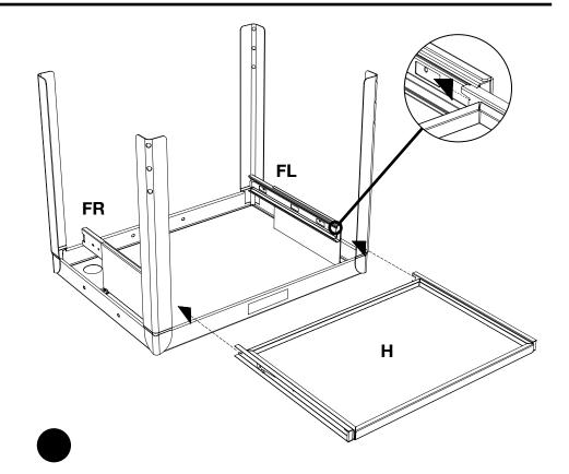
Collect parts: **H**. Align the pullout shelf **H** runner so that the runner snaps into place into the **FL** & **FR** brackets. Pull the shelf out to make sure it is fully seated. Tighten screws **A** and nut **C**. Pullout keyboard shelf assembly is now complete.
