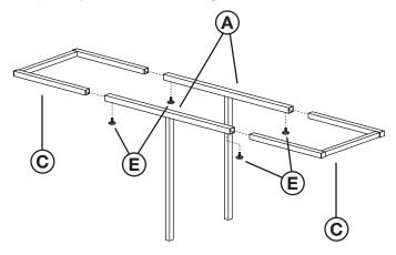
**4.** Slide Upper Frames into Lower Frames. Adjust to paper size. Insert setting knobs into holes and tighten.
