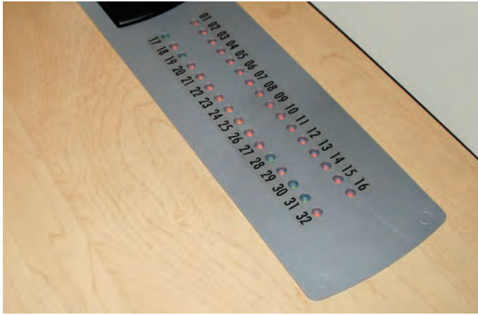
LED Status Display – Shows The State of Each Charging Device
